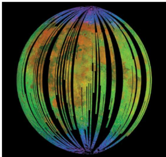
**Left:** MDL's e-beam fabricated convex grating used in the Moon Mineralogy Mapper (M3). **Right:** A three-color mosaic derived from the M3 near-infrared spectrometer. Orange and pink colors illustrate the distribution of iron-bearing minerals. Green represents the surface brightness at 2.4 micrometers. Blue indicates the presence of small amounts of surficial OH and H<sub>2</sub>O that are most prominent at these viewing geometries at cooler, higher latitudes.
