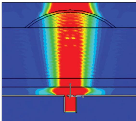
Electric field distribution of a leaky-wave antenna on a silicon lens, showing that the fields are confined to a narrow angle.
