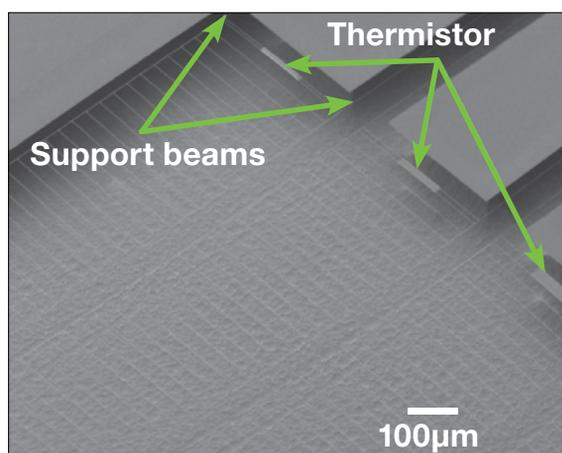
Micrograph of a segment of a 1D TES array being developed for the BLISS instrument on the Japanese SPICA mission. The TES thermistors are on  $300\ \mu\text{m} \times 2000\ \mu\text{m}$  silicon nitride absorbers, suspended (for thermal isolation) with support beams  $1000\ \mu\text{m}$  long  $\times$   $0.25\ \mu\text{m}$  thick  $\times$   $0.4\ \mu\text{m}$  wide.
