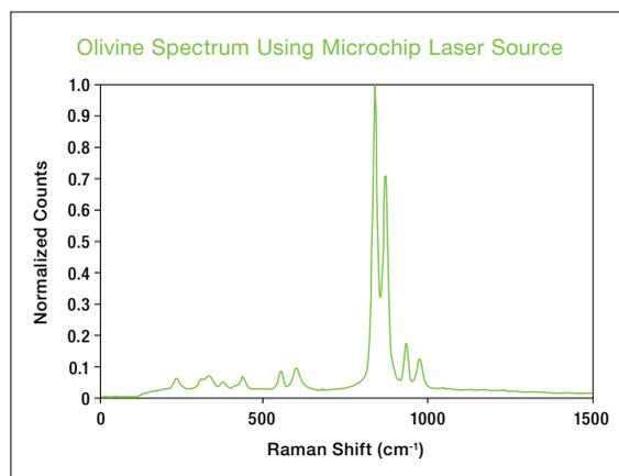
Raman spectrum of a peridotitic olivine (fosterite) acquired using a Raman spectrometer with a VLOK microchip laser integrated within a Raman probe-head. The microchip was end-pumped with 808-nm-wavelength light supplied from a multimode optical fiber.
