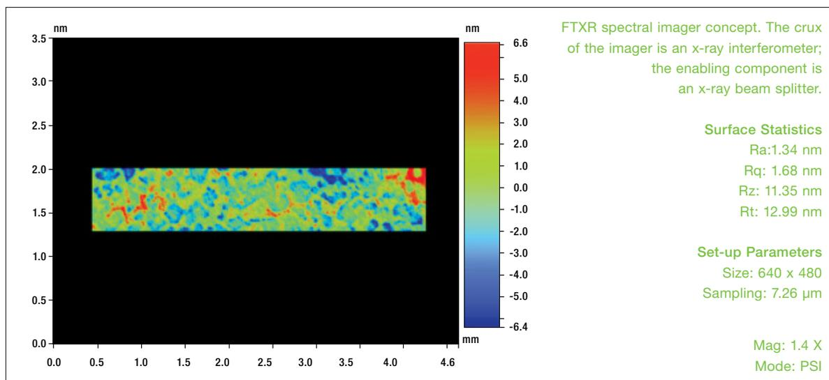
we have prepared membrane beam splitters that meet specifications on surface flatness in the VUV spectral region (up to 100 eV) — something that has eluded other researchers for years — and incorporated them into a proof-of-concept Mach-Zehnder type interferometer. The microfabrication process is being further improved to meet higher specs to facilitate wave coherence at higher x-ray energy (up to 280 eV, carbon
