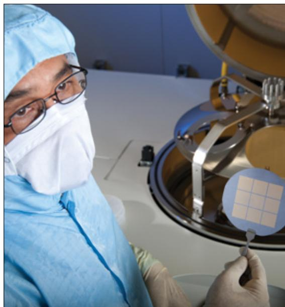
A 4-inch GaSb wafer with nine megapixel LWIR superlattice focal planes in the process of being loaded into an indium evaporator. It deposits the indium bumps on infrared detector arrays and silicon readout integrated circuits for the focal plane array hybridization process.
