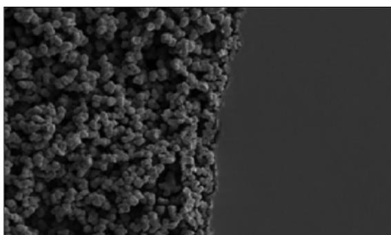
Scanning electron microscope images of microchannel cross-sections filled with porous polymer monoliths used as microcapillary electrochromatography columns on-chip.
