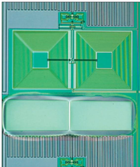
Section of a 16-element MSQUID array.
