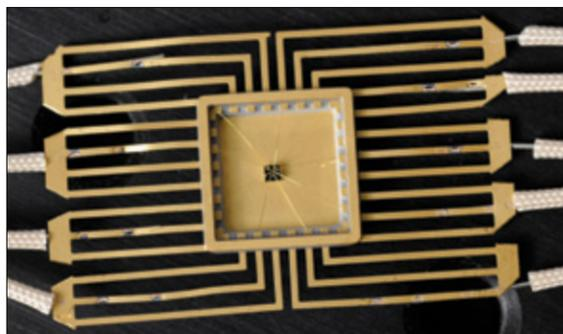
GaN MOS HEMT (metal-oxide-semiconductor high electron mobility transistor) developed for high temperature (>450 °C) operation and radiation hardness (2 Mrad).
