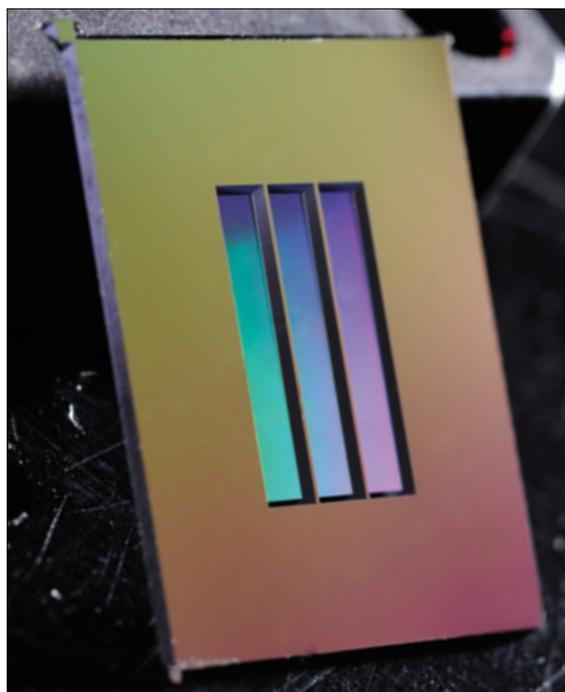
Beam-splitting mirrors consist of 200-nm-thick SiN films perforated with a large number of very small (3 mm x 15 mm) holes within a thick Si frame.
