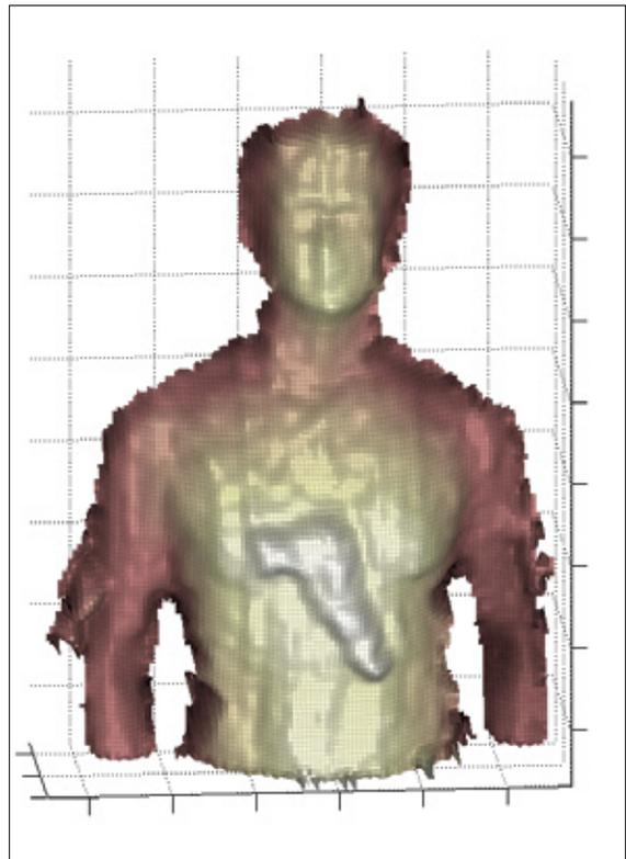
THz radar imagery reveals the presence of a replica handgun concealed underneath a shirt at a 4-meter standoff distance. Recently, the radar's imaging time was shortened by a factor of 50 and its standoff range increased from 4 to 25 meters.
