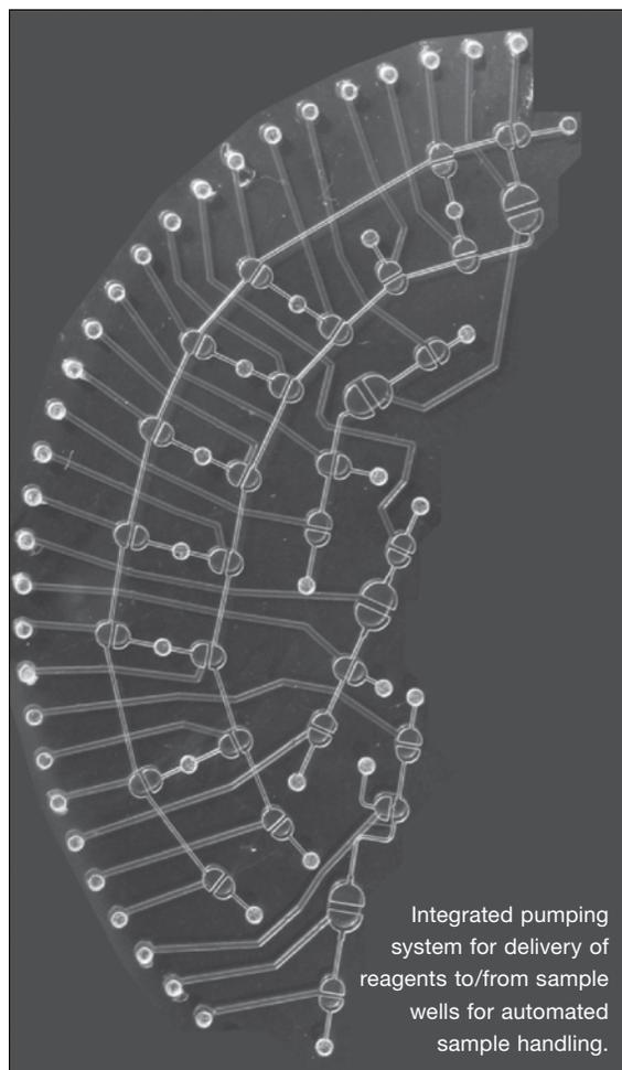
Integrated pumping system for delivery of reagents to/from sample wells for automated sample handling.
