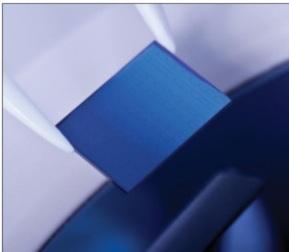
An in-process GaSb-based laser diode wafer with a silicon nitride ridge-patterned mask for dry etching in a chlorine ICP. The mask is patterned for 8, 10, 12, and 14  $\mu\text{m}$  ridges.
