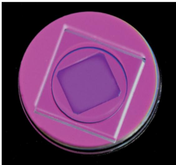
This microchip laser can be end-pumped by an 808 nm laser directly or via a fiber to provide the 532 nm wavelength light needed for a planetary Raman spectrometer.
