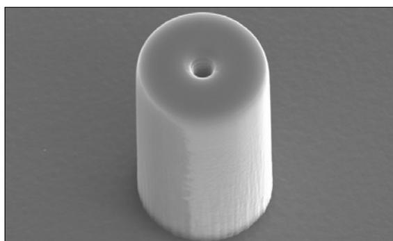
Scanning electron microscope image of a micromachined nozzle used for nanoelectrospray ionization mass spectrometry detection.
