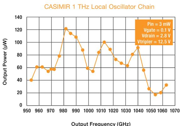
A 950–1050 GHz LO chain based on a 3x3 implementation developed for the Casimir instrument on SOFIA (PI: Jonas Zmuidzinas).
