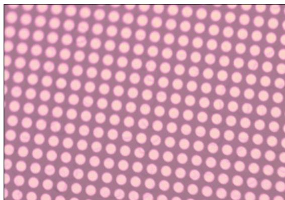
Left: Quantum efficiency of III-N arrays as a function of bias showing high QE and excellent visible light rejection. Right: Array of III-N diodes produced for process and growth optimization.
