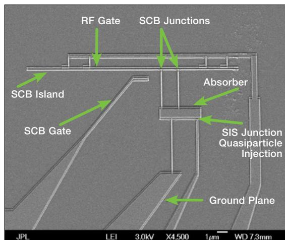
Micrograph of a detector structure used to demonstrate a proof of concept of a quantum capacitance detector. Quasiparticles from a current-biased SIS junction injected into an absorber simulate an optical signal. The quantum capacitance in the single Cooper-pair box (SCB) is proportional to the number of quasiparticles. In this first proof of concept, sensitivity better than MKIDs was demonstrated, and in principle sensitivity comparable to or better than TESs is achievable.
