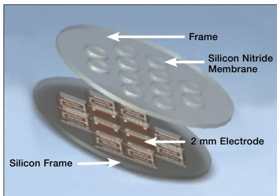
New approach that permits the deposition of reactive thin films within the sensor package directly before array deployment.
