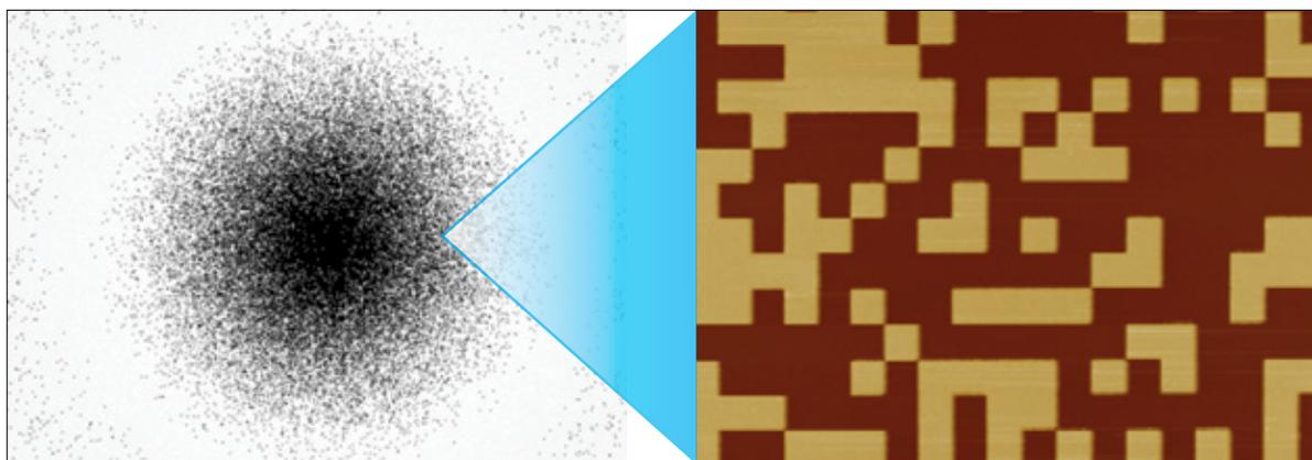
Transmission photograph and atomic force microscope scan of a half-tone occulting mask composed of near-wavelength-sized e-beam fabricated aluminum squares. The granularity is smoothed out when integrated over the image of the star.
