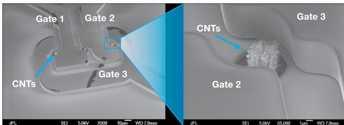
Left: SEM micrograph shows single-bundle device as fabricated. Right: Close-up view of the device.
