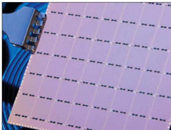
DEMOCAM2 array for a submillimeter camera for the Caltech Submillimeter Observatory. Each pixel consists of a slot array antenna. The power received by each of these antennas is split into 3 bands (1.3 mm, 1.1 mm, and 850  $\mu\text{m}$ ) and detected by a separate MKID. A single microwave feedline is used for reading out the entire array.
