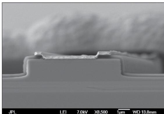
A scanning electron microscope image of a fully processed, 8  $\mu\text{m}$  laser ridge designed to emit light at 3.1  $\mu\text{m}$ .
