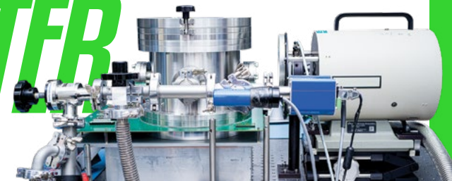
Picture of the vacuum testbed used to measure the performance of the FPM. A blackbody (right) shines IR radiation through a window into the vacuum chamber where the FPM is mounted. Electronics not shown control the FPM and record the signals from each of the pixels.
