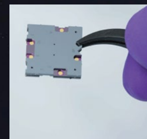
Reduced size, mass, and power in spacecraft environmental monitoring (involving MDL developed high-pressure microelectromechanical systems [MEMS] microvalves, semiconductor lasers and associated systems)
