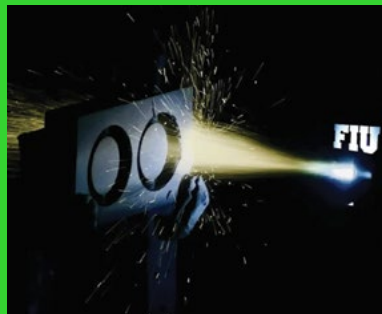
In the Plasma Forming Laboratory, high-temperature plasma is sprayed on metallic samples to deposit FIU's coating material.
