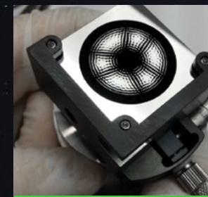
Roman Space Telescope Cronograph Instrument (CGI) (2027 launch) (with MDL supplied Diffractive Optics and occulting spots, light trapping surfaces, precision slits, mirror control actuator elements, coatings, etc.)
