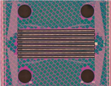
The flight 64 x 8 element thermopile array, which has a new 'diamond' bulk micromachined design to remove most of the silicon from the substrate to reduce the electrical capacitance to ground. This reduction lowers the noise by 30-50%.
