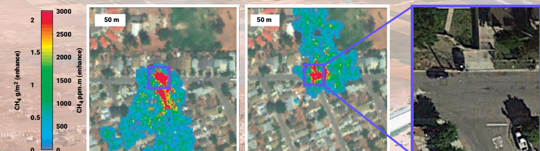
Mitigation of neighborhood natural gas leak using airborne measurements.
