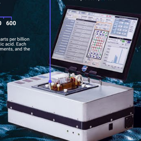
The Chemical Laptop: a fully automated instrument for performing analysis of organics by microchip electrophoresis.
