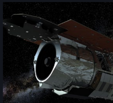
Roman Coronagraph Instrument (CGI): HLC or PIACMC designs with e-beam gray scale and MDL black silicon, and deformable mirror metallization/lithography.
